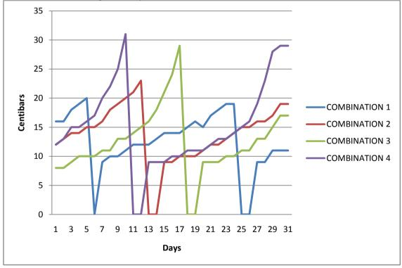
From the experimental analysis it is found that irrigation frequency of plants changes with different combination.Combination having higher bentonite requires less frequent irrigation while those having lower are irrigated more. This is because the infiltration of water reduces and water holding increases due to the addition of bentonite clay.
